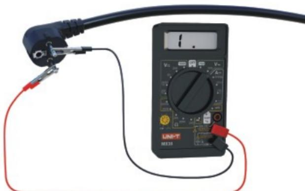
Measurement of the heating core's resistance
