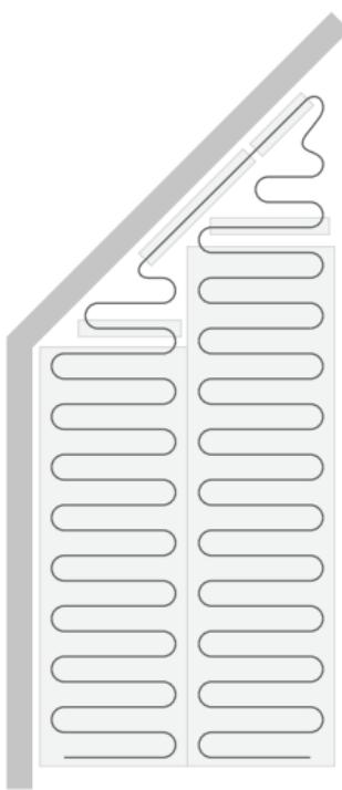
In places where the heating mat cannot be laid properly, it is possible to remove the heating mat's cable from the mesh or cut the mesh into narrow strips, so as to enable the desired cable arrangement.
