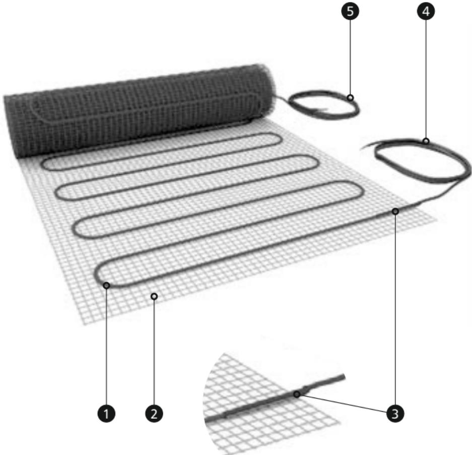
The ELEKTRA MD heating mats are 3.9 mm thick and are provided with a 4.0 m long cold tail at one end and a joint at the other.
