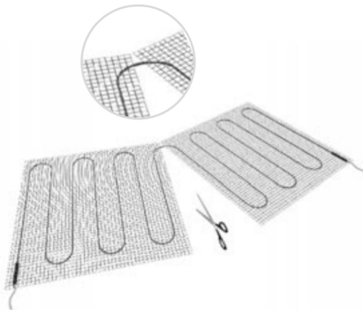
While planning the heating mat's layout, consider the cuts needed to achieve the desired layout.
