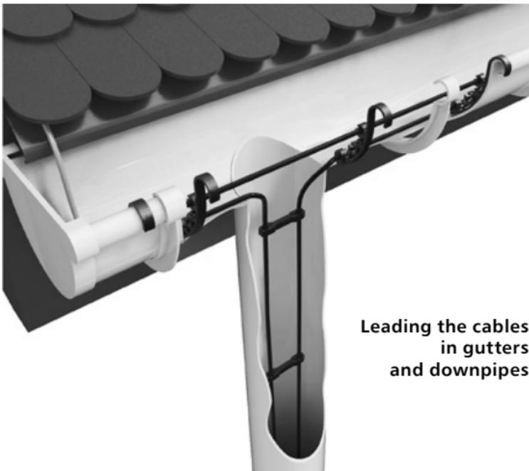
Protect the joining spot of the gutter and downpipe with a flexible cable support to prevent possible damage to the cable.
