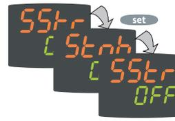
The label and the current status of the function will be displayed. To scroll the available functions, use the 'set' key.
